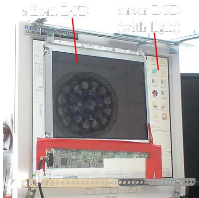
Fig. 2. The developed volumetric display. The rear LCD is an I-O DATA product LCD-AD19H. The front LCD is a DISIGN product R120F00-M1TR, that is sold by the usage in outdoor.
