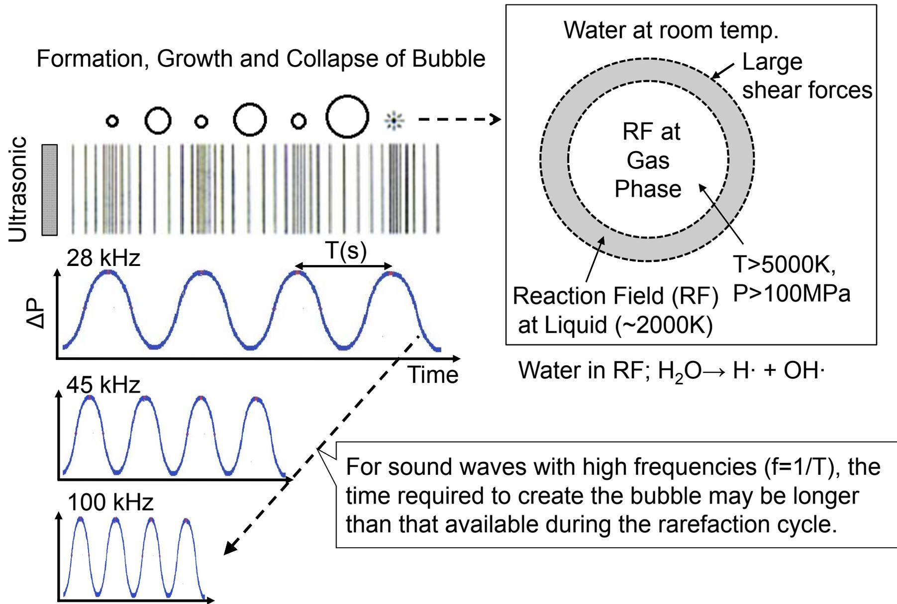
Fig.7 Schematic representation of bubble formation, growth and collapse under ultrasonic irradiation, in which hot spot induces radical reactions.
