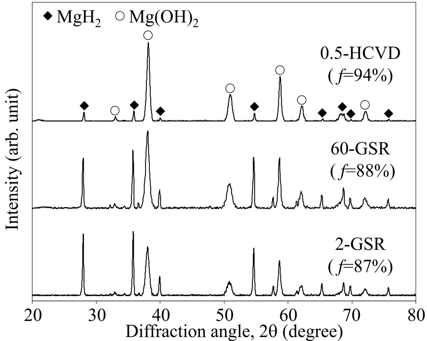
Fig. 6 X-ray diffraction patterns of three sonicated samples at ultrasonic frequency of 28 kHz, which were recovered at 7.2ks.
