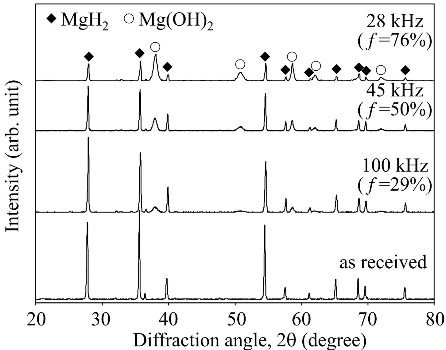
Fig. 4 Effect of ultrasonic frequency on the remaining sample of 60-GSR- $\text{MgH}_2$  at 7.2ks. The XRD pattern of each sample shows that the smaller frequency caused the more  $\text{Mg(OH)}_2$  as product.
