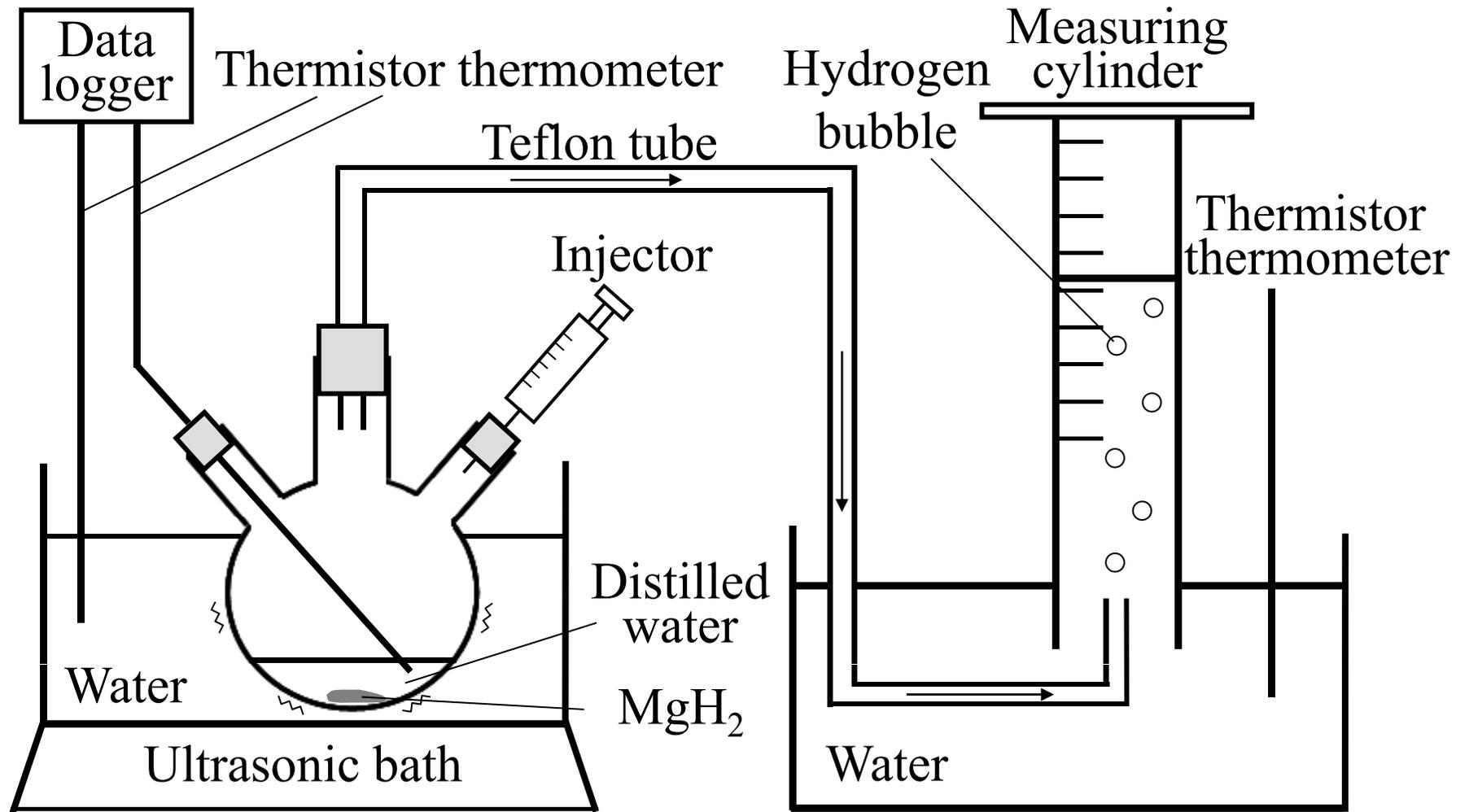
Fig. 2 Schematic diagram of the experimental setup for the hydrolysis of  $\text{MgH}_2$ , in which the experiments started by adding distilled water of  $5 \text{ cm}^3$  to  $\text{MgH}_2$  samples of  $0.1 \text{ g}$  at  $25 \text{ }^\circ\text{C}$  and the hydrogen evolution was monitored by a water substitution method.
