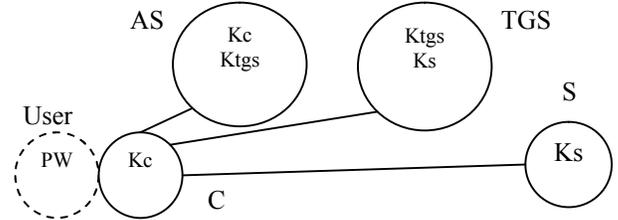
Figure 10. Kerberos configuration
