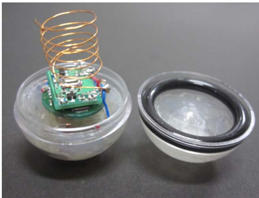
Fig. 1 Appearance of sensor particle with a built-in sensor system.
