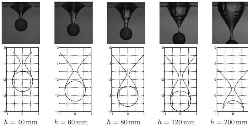
**Fig. 1** Air cavity shapes, at pinched off, formed by the water entry of a superhydrophobic low-density sphere ( $d_p = 12.7$  mm and  $\rho_p = 851$  kg/m<sup>3</sup>). *Top* photograph, *Bottom* analytical model of Duclaux *et al.* (2007).
