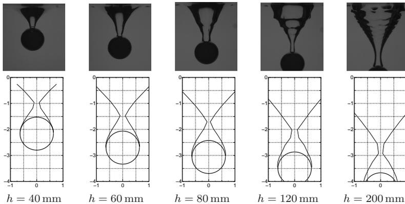
**Fig. 2** Air cavity shapes, at pinched off, formed by the water entry of a superhydrophobic low-density sphere ( $d_p = 12.7$  mm and  $\rho_p = 920$  kg/m<sup>3</sup>). *Top* photograph, *Bottom* analytical model of Duclaux *et al.* (2007).
