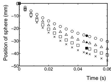
**Fig. 5** Position of a sphere ( $d_p = 12.7 \text{ mm}$  and  $\rho_p = 851 \text{ kg/m}^3$ ) entering into water. *Circle*:  $h = 50 \text{ mm}$ , *Triangle*:  $h = 80 \text{ mm}$ , *Square*:  $h = 120 \text{ mm}$ , *Cross*:  $h = 160 \text{ mm}$ . Data at the pinch-off event is indicated as solid/bold symbol.
