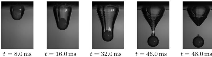
**Fig. 4** A video sequence of the water entry of a hydrophobic sphere from the onset of the impact to the pinch-off in the case of  $d_p = 12.7 \text{ mm}$ ,  $d_p = 851 \text{ kg/m}^3$  and  $h = 160 \text{ mm}$ .
