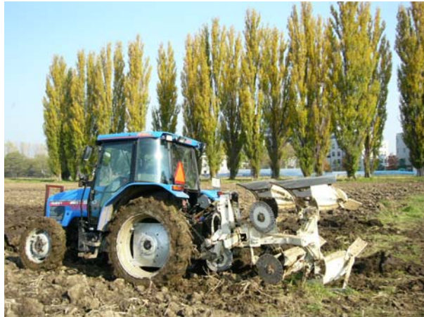
Fig. 6-17. Two-furrow Moldboard Plow of Reversible Type (Sugano-Noki, TROY1921DC).
