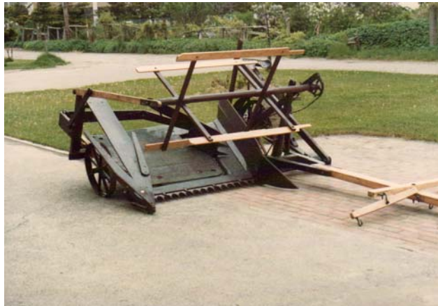
Fig. 6-5. Wheat Reaper (Re-build Specimen).
