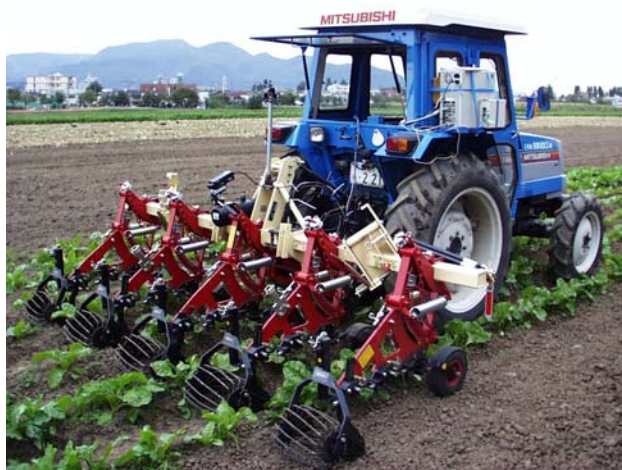
Fig. 6-22. Weeding Machine (Nichinoki-Seiko, NAK-5).
