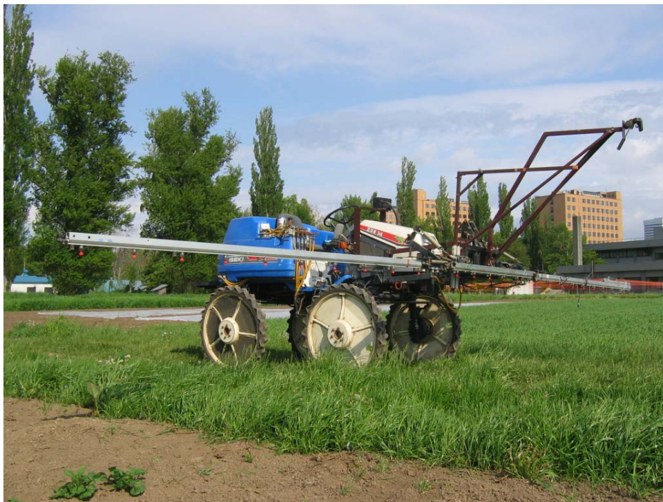
Fig. 6-21. Utility Vehicle (Sprayer Version, Iseki JK-14).
