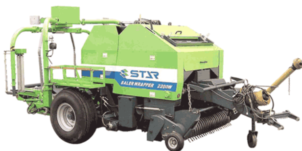
Fig. 6-29. Roll Baler with Rapping Machine System.
