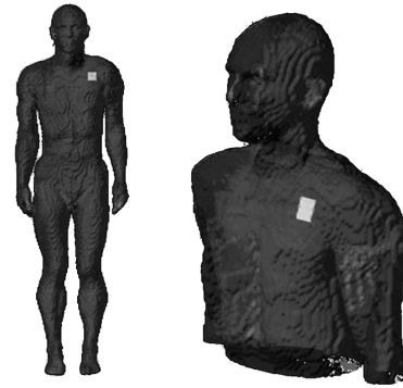
Fig. 7 Representation of the phantom model with pacemaker.
