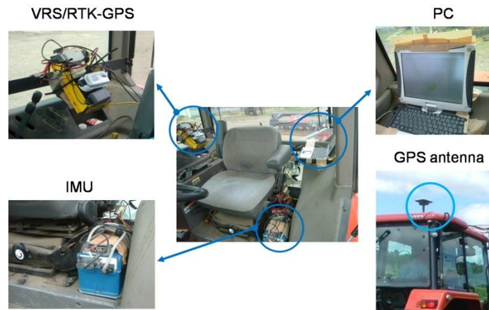
Fig. 2 Installation of the tractor vibration data-acquisition system.
