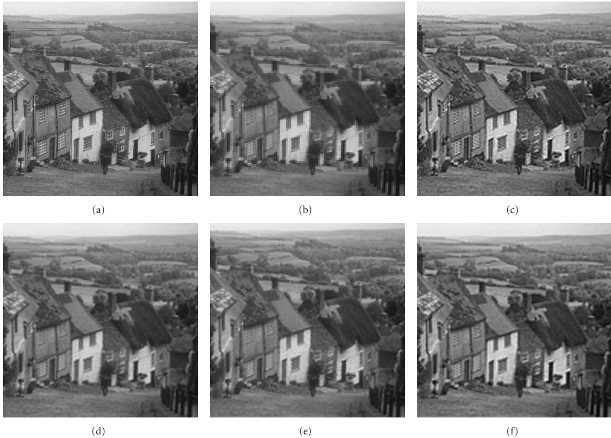
FIGURE 5: Subjective performance comparison between the proposed method and the conventional methods (the magnification factor was set to four): (a) original HR image “Goldhill” ( 512 \times 512 pixels), (b) LR image ( 128 \times 128 pixels), (c) HR image estimated by the proposed method, (d) HR image estimated by the interpolation using Lanczos filter, (e) HR image estimated by [10], and (f) HR image estimated by [21].
