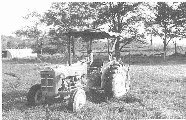
Fig. 2 Tractor used to measure vertical acceleration of tractor body and tractor seat.
