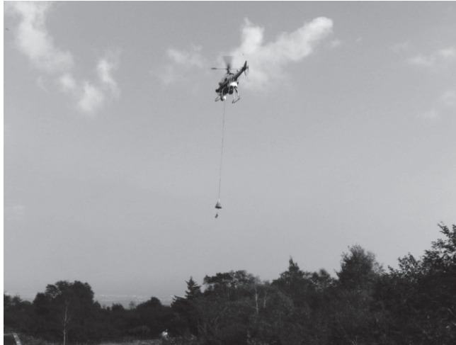
Fig. 5. Unmanned helicopter operating magnetic survey. Magnetic sensor is suspended with the wire of 4.5 m long.
