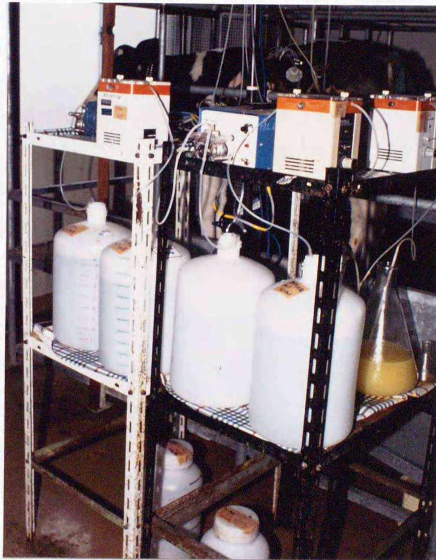
Plate 1. The 10-wk-old calf nourished by intragastric infusion: (a) arrangement of infusion tubes. (b) peristaltic pumps and infusion reservoirs.
