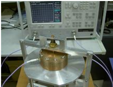
Fig.8 Apparatus of the perturbation resonator method
