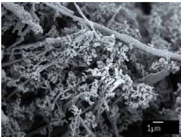
Fig. 5 SEM image of tantalum titanium powder reduced by Ca. The needle-like chained structure (“branch”) is characteristic in the morphology such as broccoli.
