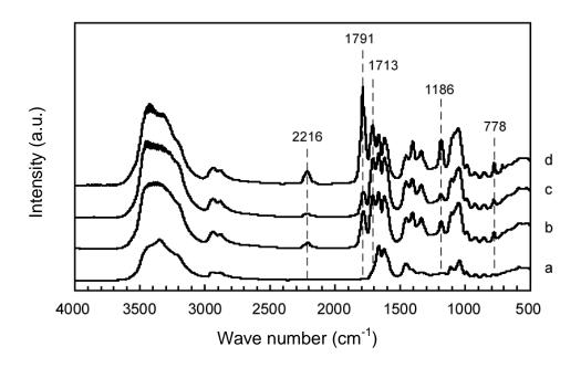
**Fig. 4.** FTIR spectra collected in the presence and absence of Zn-containing solid catalysts. (a) glycerol + urea, (b) glycerol + urea + ZnO, (c) glycerol + urea + SM(Zn), and (d) glycerol + urea + HT(Zn).
