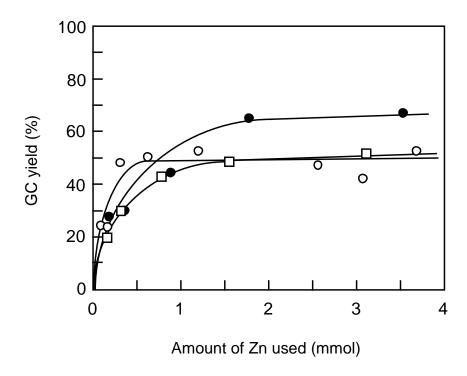
**Fig. 2** The yield of glycerol carbonate as a function of the amount of Zn included in the catalyst used. ( $\circ$ ) ZnO, ( $\square$ ) SM(Zn), and ( $\bullet$ ) HT(Zn).
