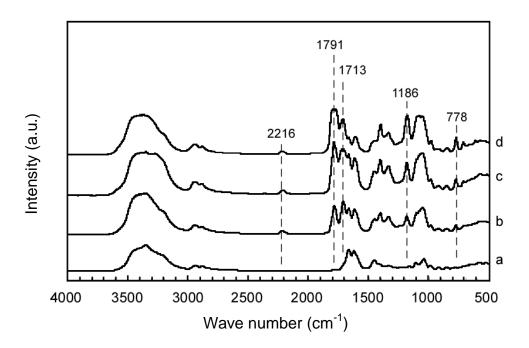
**Fig. 5.** FTIR spectra collected in the presence and absence of Zn-containing homogeneous catalysts. (a) glycerol + urea, (b) glycerol + urea +  $ZnCl_2$ , (c) glycerol + urea +  $(CH_3COO)_2Zn$ , and (d) glycerol + urea +  $ZnSO_4$ .
