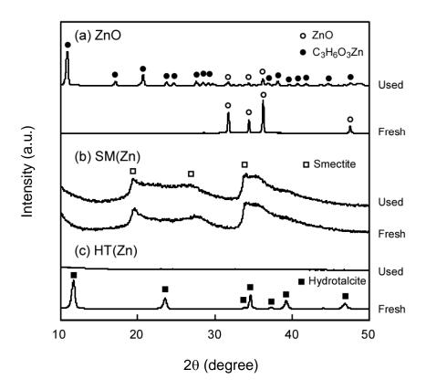
**Fig. 1.** XRD patterns of Zn-containing solid catalyst samples used: (a) ZnO, (b) smectite, and (c) hydrotalcite before and after activity measurements in glycerol carbonate synthesis
