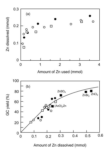
**Fig. 3.** (a) Relationship between the amount of Zn species dissolved and the initial amount of Zn included in the parent catalysts. (b) Relationship between the yield of glycerol carbonate (GC) and the amount of Zn species dissolved in the liquid phase. ( $\circ$ ) ZnO, ( $\square$ ) SM(Zn), ( $\bullet$ ) HT(Zn) and ( $\blacksquare$ ) zinc salts.
