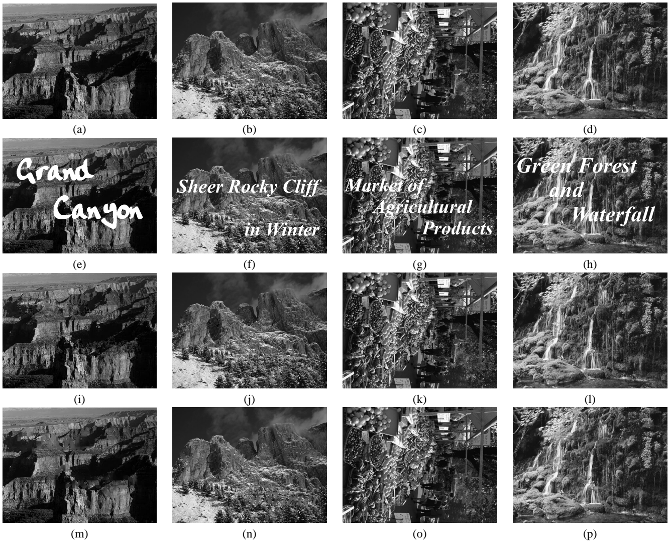
Fig. 4. (a)–(d) Original images ((a) 480 \times 359 pixels, (b) 640 \times 480 pixels, (c) 480 \times 640 pixels, (d) 640 \times 480 pixels), (e)–(h) Corrupted images of (a)–(d) ((e) 8.9% loss, (f) 5.4% loss, (g) 6.2% loss, (h) 6.7% loss), (i)–(l) Reconstruction results of (e)–(h) by the proposed method, (m)–(p) Reconstruction results by the conventional methods ((m) Reference [3], (n) Reference [7], (o) Reference [8], (p) Reference [9]). All of these images are 8-bit gray levels. In order to save the pages, we show the rotated images for (c), (g), (k) and (o). Furthermore, the numbers of training patches were respectively 107, 215, 209 and 218 in (e)–(h), and the patch size was set to 31 \times 31 pixels.
