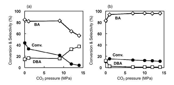
**Fig. 1.** Influence of  $CO_2$  pressure on total conversion and product selectivity in hydrogenation of BN in the absence (a) and presence (b) of  $H_2O$  using  $Pd/Al_2O_3$  at 323 K and at a  $H_2$  pressure of 2 MPa for 4 h.
