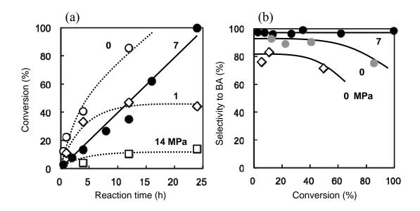
**Fig. 2.** (a) Time profiles of total conversion in hydrogenation of BN in the absence  $(\circ, \Diamond, \Box)$  and presence  $(\bullet)$  of  $H_2O$  (5 cm<sup>3</sup>) and at  $CO_2$  pressures given. (b) The relationship between BA selectivity and total conversion in the absence  $(\diamond)$  and presence  $(\bullet, \bullet)$  of  $H_2O$  (5 cm<sup>3</sup>) and at  $CO_2$  pressures given.
