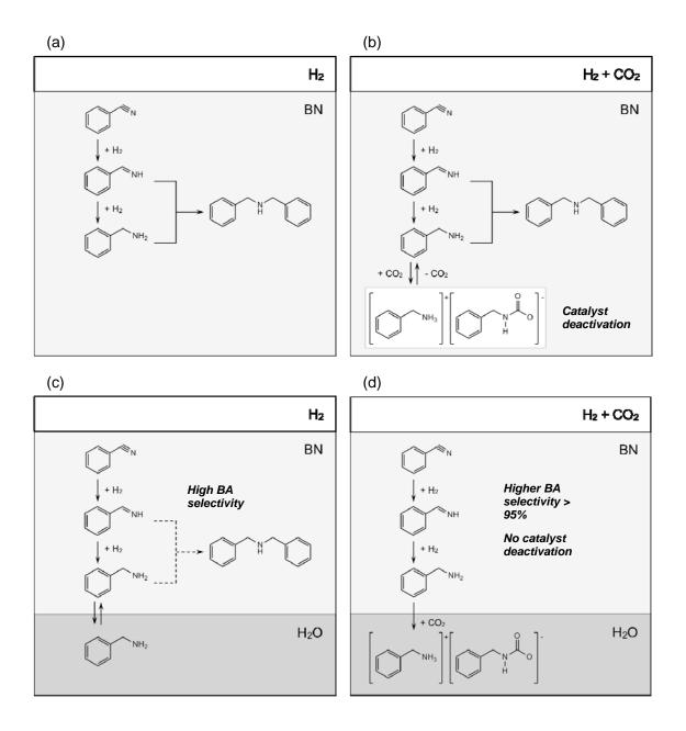
**Fig. 5.** Illustration of features of BN hydrogenation reactions in four different multiphase media in the absence and presence of CO<sub>2</sub> and/or H<sub>2</sub>O. The solid catalyst phase is not displayed herein.
