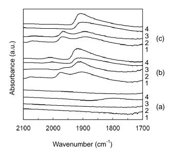
**Fig. 4.** *In situ* high-pressure FTIR spectra of CO adsorbed on  $Pd/Al_2O_3$  after reduction (a), after exposure to atmospheric CO for 10 min (b), and after purging with  $N_2$  (c) in the absence (1) and presence of  $H_2O$  (2), BN (3), and  $H_2O + BN$  (4).
