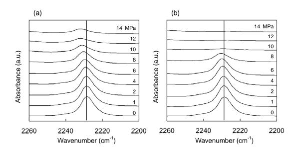
**Fig. 3.** *In situ* high-pressure FTIR – ATR spectra collected at 323 K for liquid BN (a) and for H<sub>2</sub>O dissolving BN (b) compressed by CO<sub>2</sub> at pressures given
