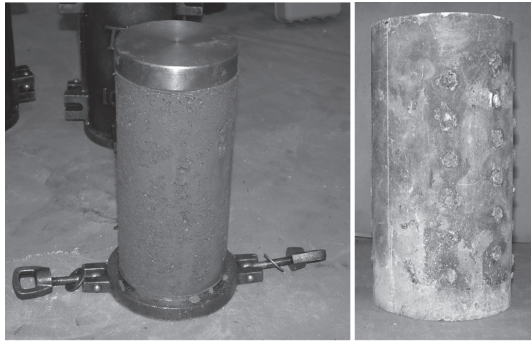
(a) Base concrete (normal strength) (b) Shotcrete Fig.1 Examples of the specimens before compression.
