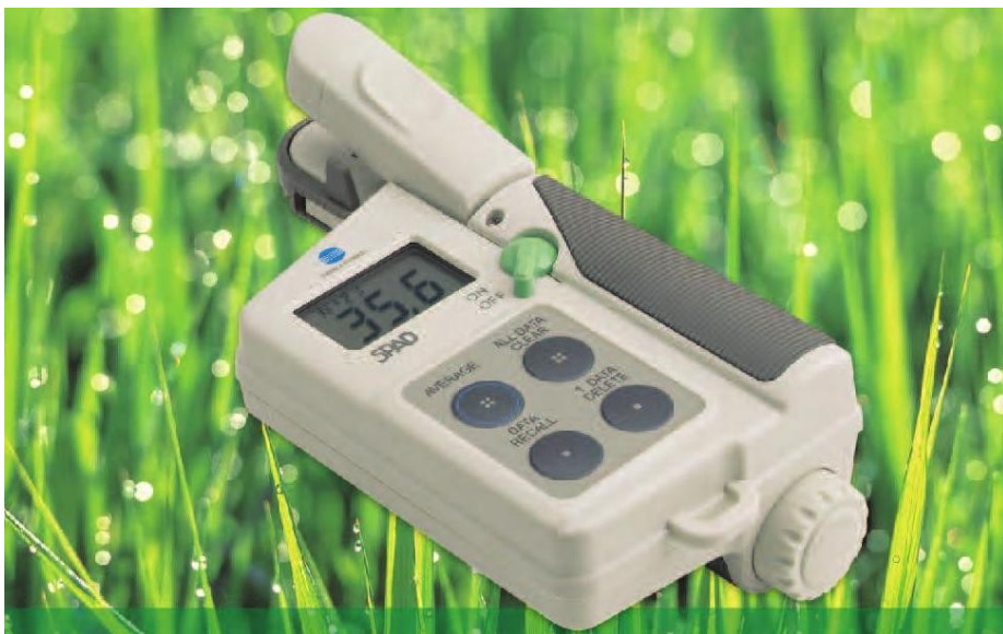
Fig. 3.3 SPAD merer that measures SPAD value
