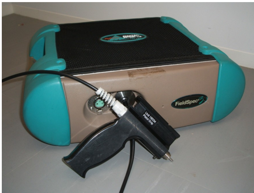
Fig. 3.5 Spectroradiometer 3 (field spec 3) (Analytical Spectral Devices, Inc., USA)
