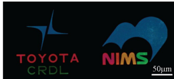
Fig. 1.7 Optical microscope image of aluminum color filter with triangular shaped holes. (Adapted from Ref. [18])
