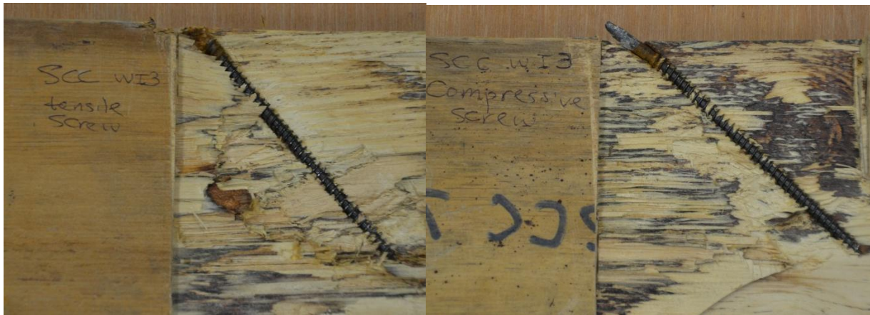
Figure 6: Opened specimen of SCC series, tensile screw (on left) and compressive screw (on right).
