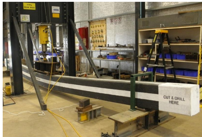
Figure 6: Glue-laminated fibre composite sandwich bridge girder.
