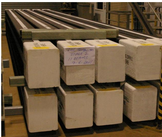
Figure 6: Glue-laminated fibre composite sandwich bridge girder.
