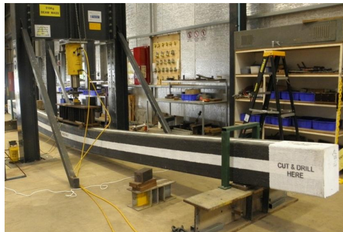
Figure 6: Glue-laminated fibre composite sandwich bridge girder.
