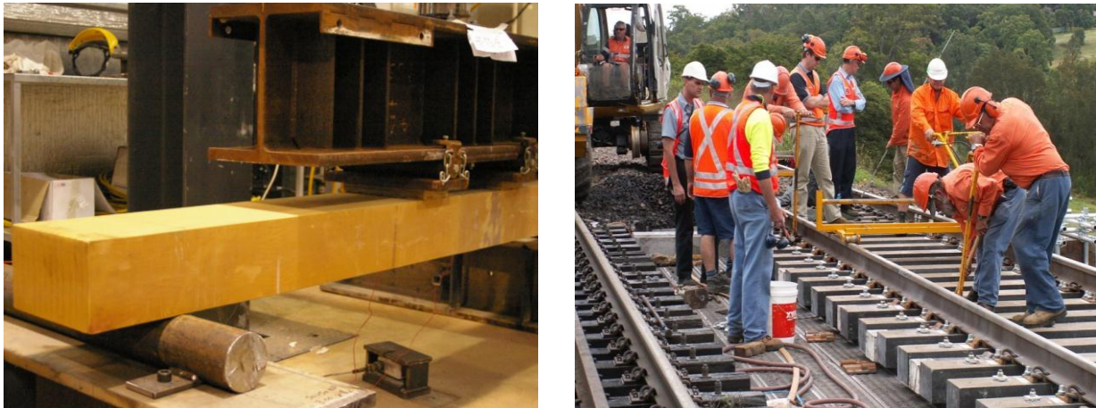
Figure 3: Glue-laminated fibre composite sandwich railway sleepers.
