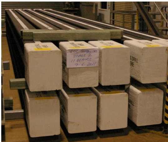
Figure 6: Glue-laminated fibre composite sandwich bridge girder.
