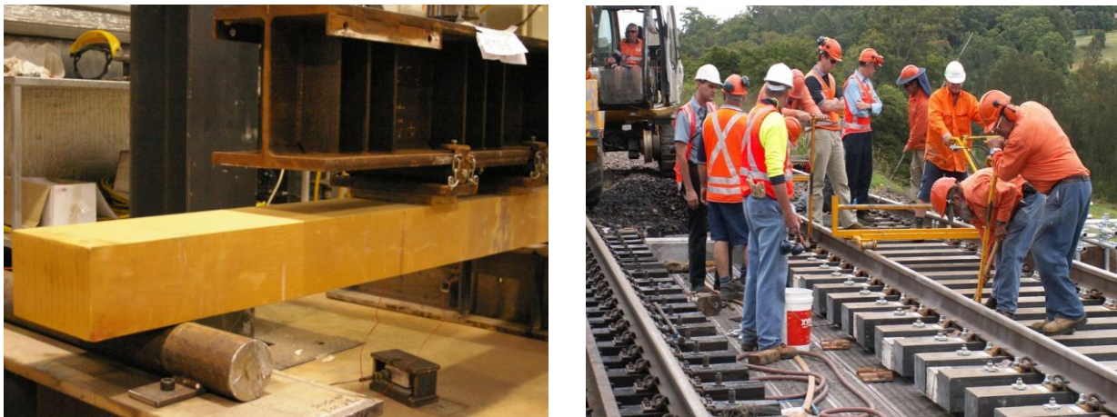
Figure 3: Glue-laminated fibre composite sandwich railway sleepers.
