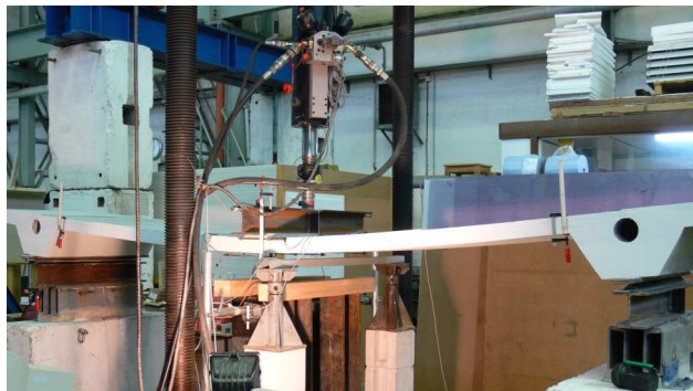
Figure 10: Full scale test to determine the bearing capacity of lateral direction
