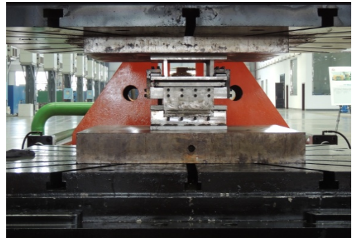
(b) Metallic isolator
