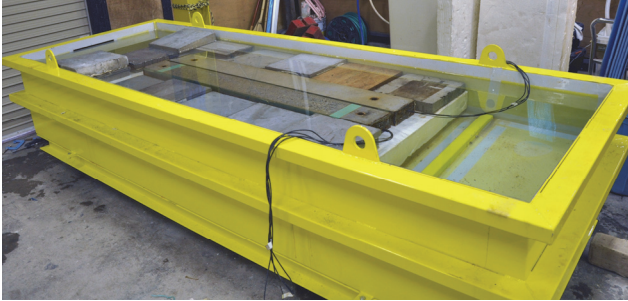
Photo 1: RC beam placed in water
