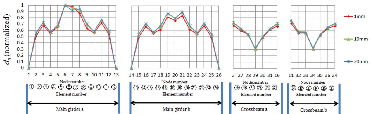
Figure 6: Damage index  $d_n$  in damage scenario A
