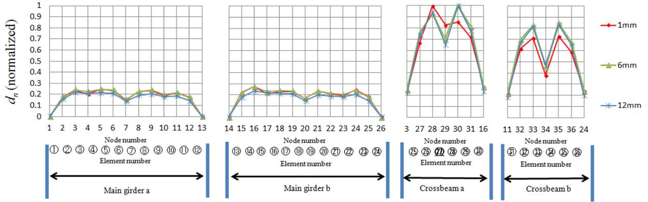
**Figure 7: Damage index  $d_n$  in damage scenario B**
