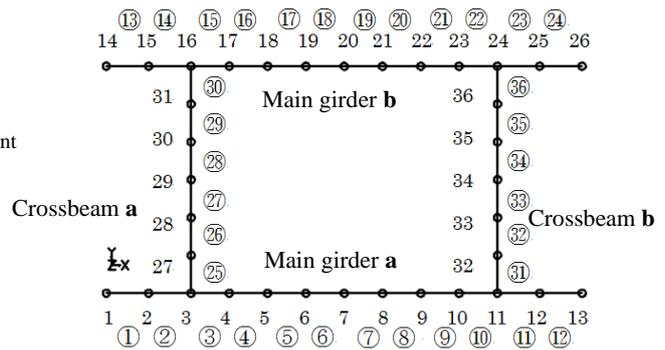
Figure 4: Node numbers and element numbers (Circled)
