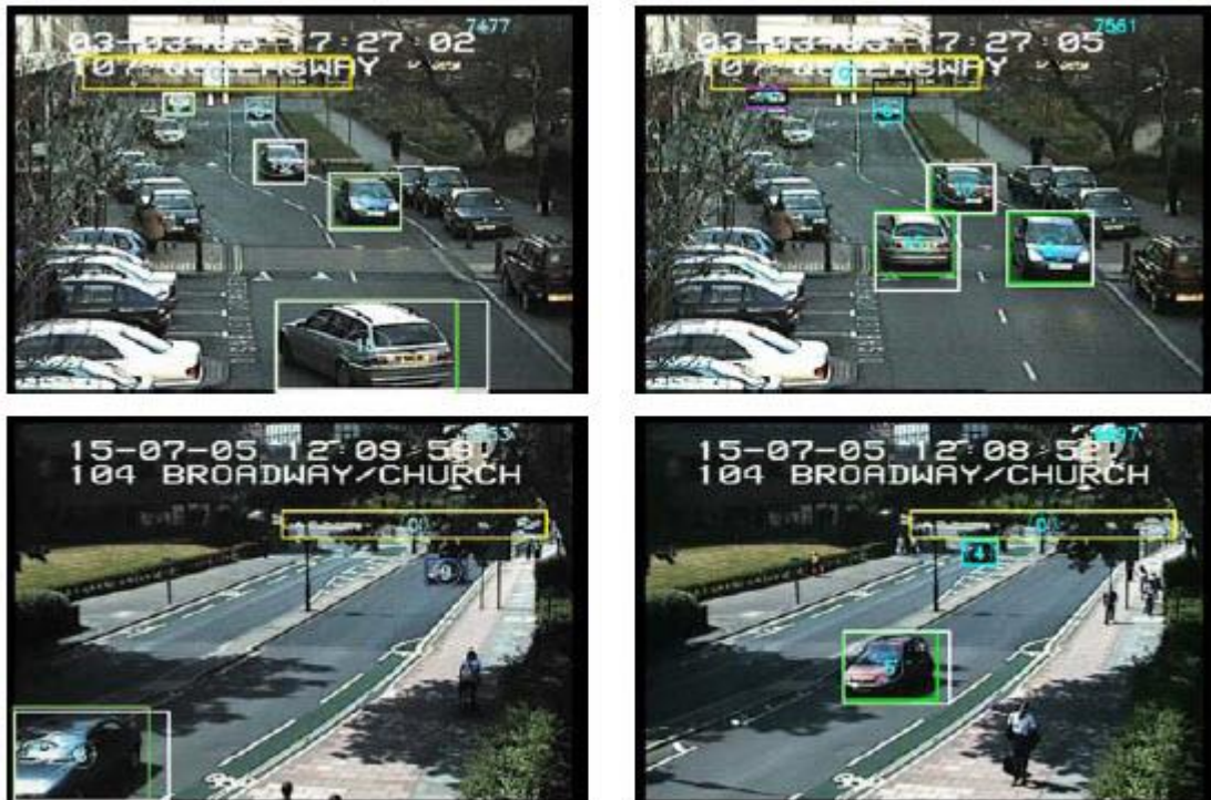
Figure 2.8 Results of vehicle tracking and detection (Yellow box: DCO (Don't Care Object), Green box: Detected ground truth, White box: Detected system output, Blue box: Missed ground truth, Black box: Detected but overlapped with DCO, Magenta box: Occluded ground truth (DCO), Cyan box: Stationary ground truth (DCO)).
