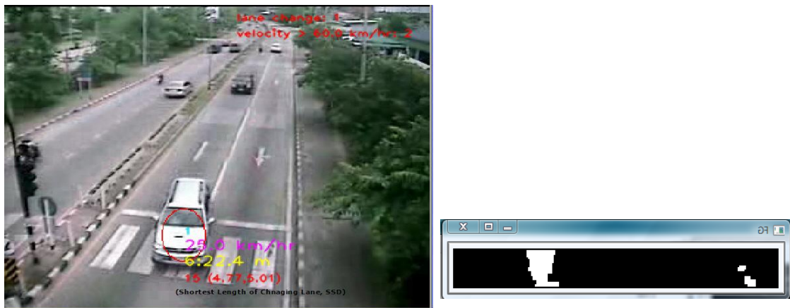
(a) Separated object frame from VDO (b) Separated object from the background
