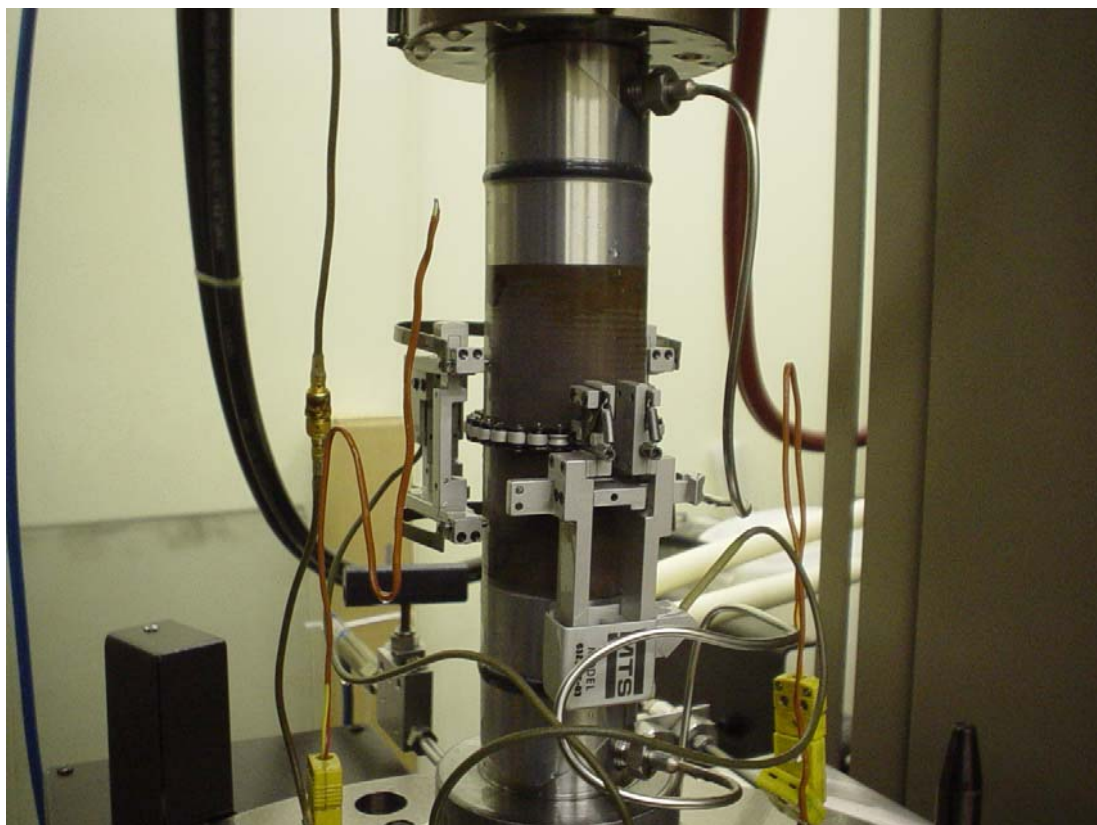
Fig. 7.11 Photograph of specimen assembly. Specimen (Horonobe mudstone) is pinched by a couple of end caps, covered with heat shrinkable tube, and attached on with extensometer, on pedestal of testing apparatus.
