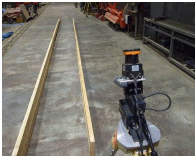
Figure 4.6 Test of laser scanner based guidance system at laboratory condition.
