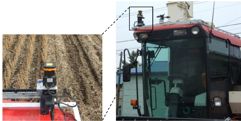
Figure 4.7 A combine harvester with the guidance system at a real soybean field.
