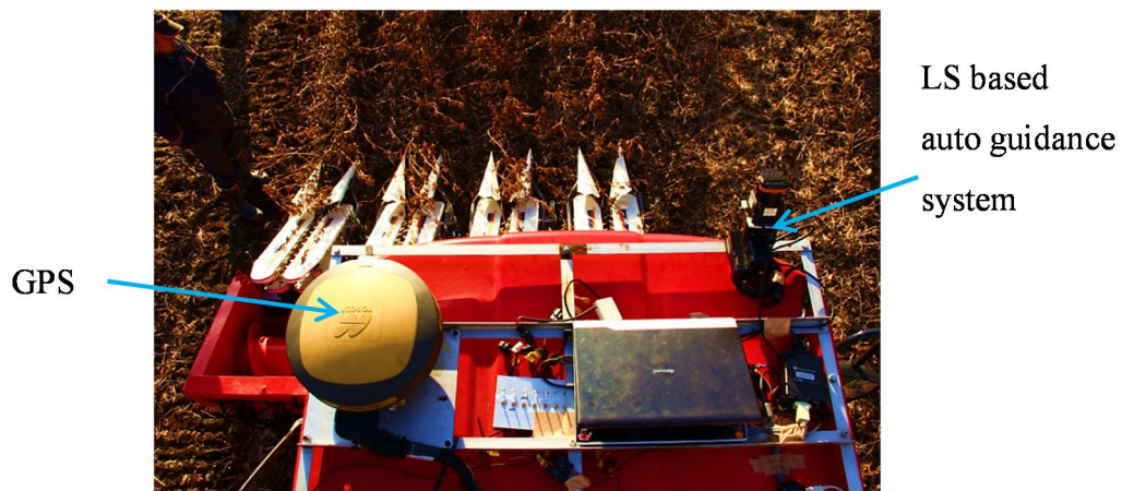
Figure 5.5 GPS and LS based auto guidance system mounted at the roof of the combine harvester.
