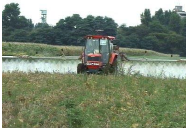
Figure 1-6 A robot tractor by using RTK-GPS and FOG (Kise et al. 2001)
