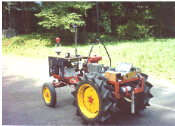
Figure 1-5 A robot tractor using a vision and a GDS sensor (Ishii et al. 1994, 1995, 1998)
