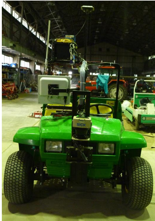
Figure 1-7 An autonomous vehicle using a 2D laser scanner (Barawid et al. 2007)
