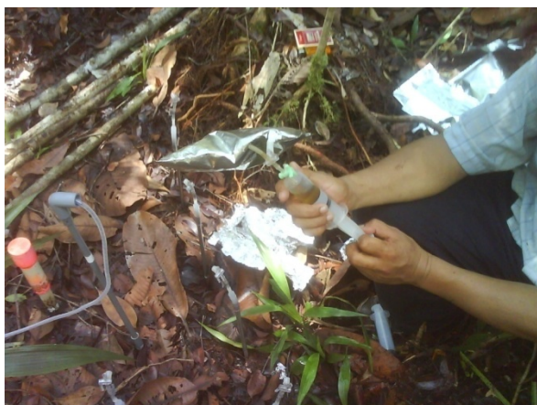
Fig. 6.1 View of the rapid equilibration method for the measurement of dissolved \text{CH}_4 and \text{N}_2\text{O} concentrations.
