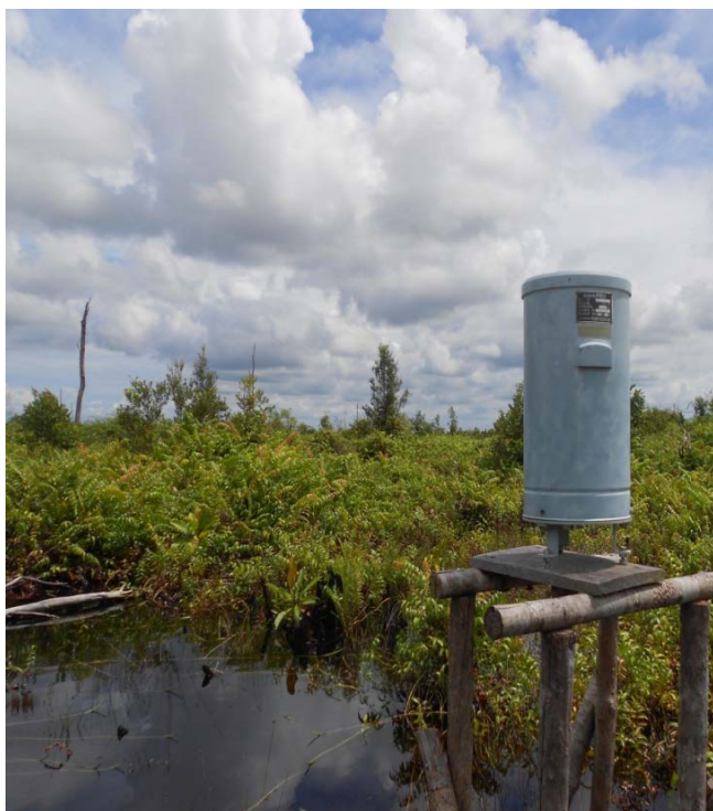
Fig. 4.1 View of the tipping bucket rain gauge settled near the base camp of Kalampangan canal.
