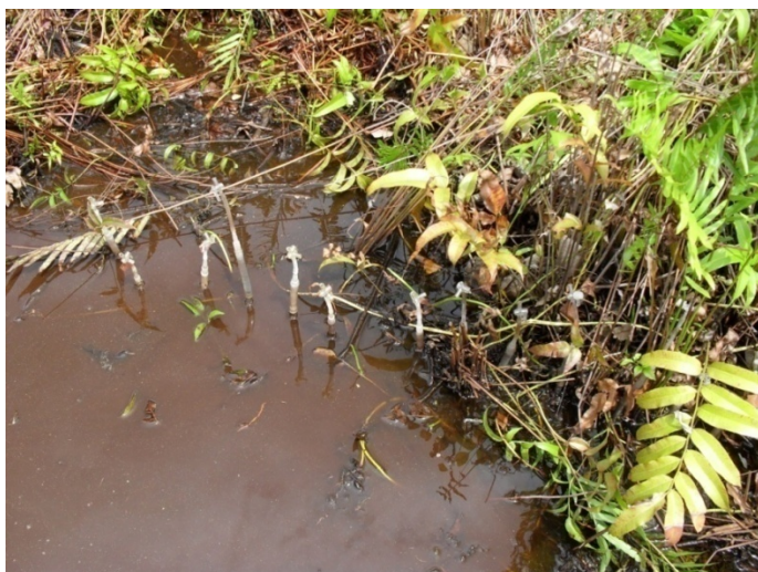
Fig. 4.4 View of a set of water samplers for pH, EC, \text{NO}_3^- , \text{NH}_4^+ , and DO measurements at the study site.
