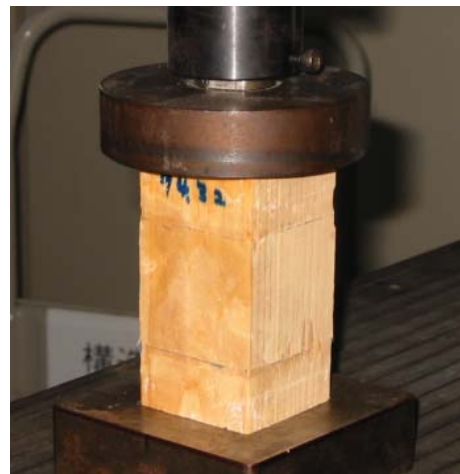
Fig. 2.3 Compressing test of decayed specimen.
