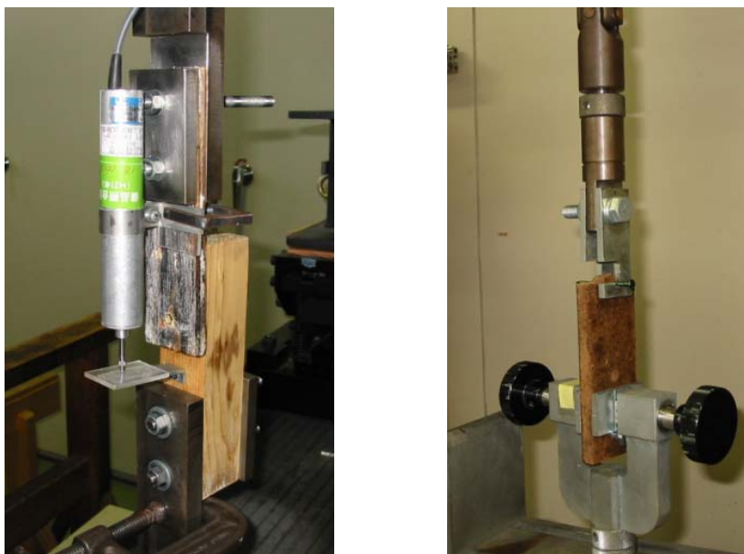
Fig. 3.2. Strength test of nailed joint (left: shearing test, right: lateral resistance test).
