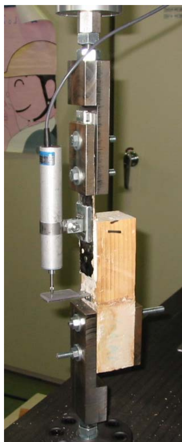
Fig. 2.4 Shearing test of nailed timber joint with a steel plate.
