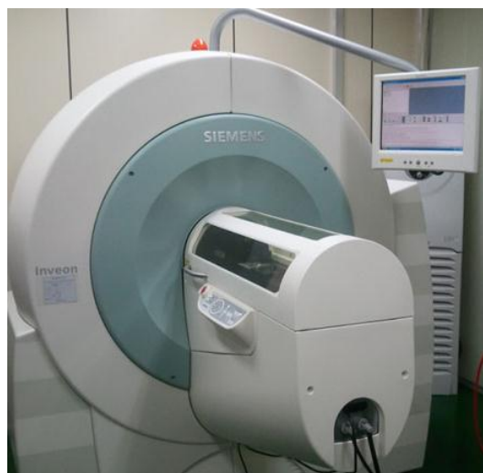
Figure 1 The SPECT component has dual head detector geometry that is mounted on a rotating gantry, Each detector head contains a 68x68 pixelated scintillator array of 2.0x2.0x10 mm NaI-(Tl) crystals with 0.2-mm gap, in combination with a position-sensitive photomultiplier readout
