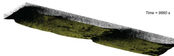
Figure 10. Visualization of the sediment particles above the bed forms for run RT01. The concentration of sediment is highest behind the crest of sharp dunes, due to the boiling effect.
