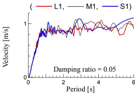
Fig. 3 Velocity response spectra of input motions.
