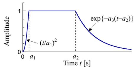
Fig. 5 Time envelope functions of input motions.
