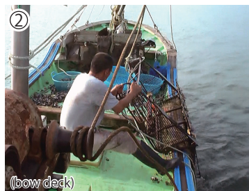
fix dredges on bulwark
