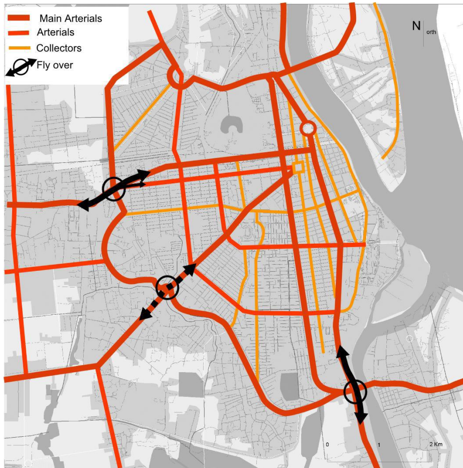
Figure 2-3: 4 central districts road network – source SYSTRA 2012
