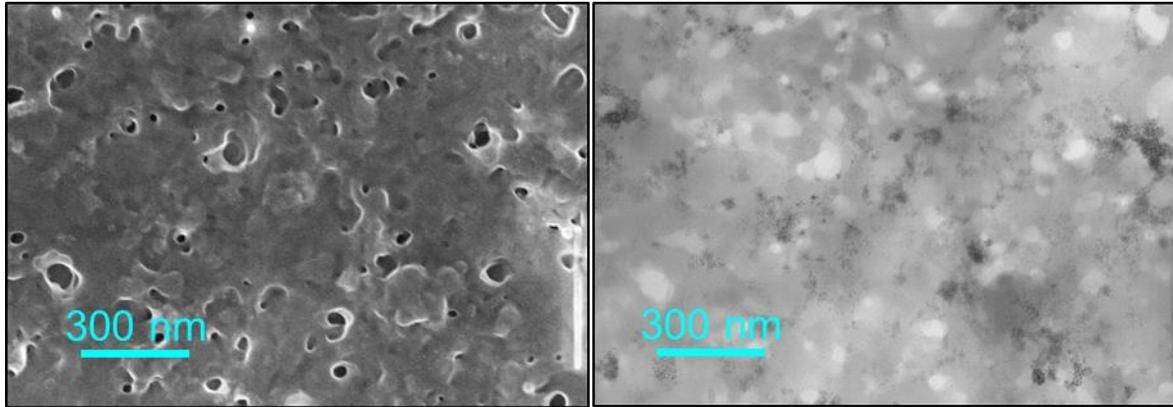
**Figure 3-10.** SE-STEM (left) and BF-STEM (right) images of Pd nanostructures from Pd4-p53Tet after omitting the pre-reduction incubation period. This control experiment suggests that the formation of the porous, coral-like materials involves a step-wise process
