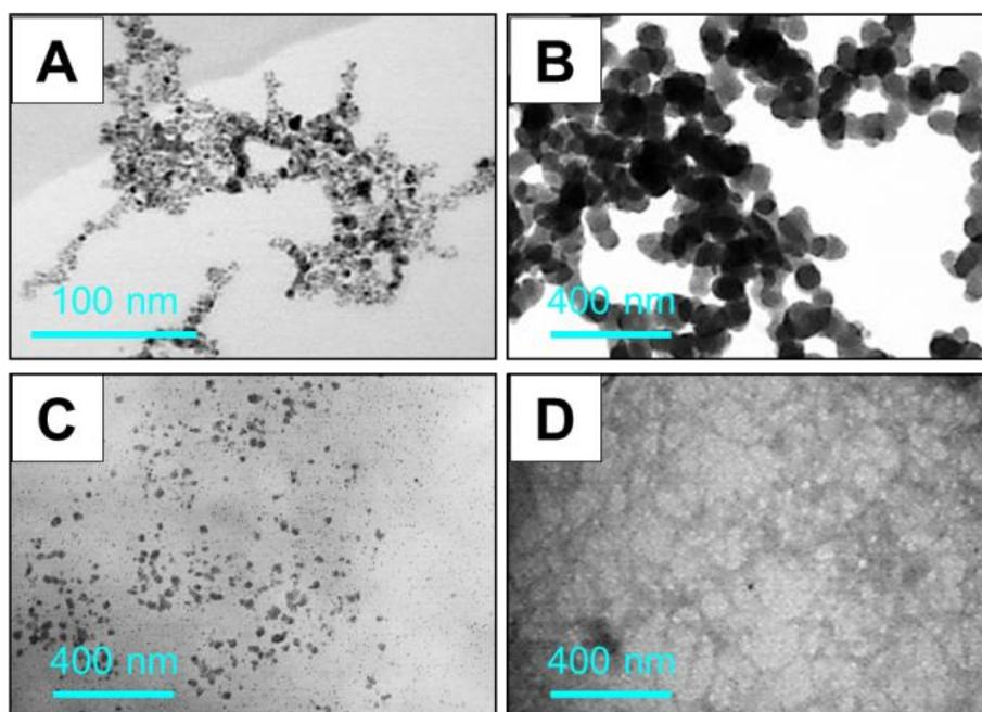
**Figure 3-7.** BF-STEM images of the Pd nanostructures prepared using peptide sequences **A)** No peptide, **B)** Pd4, **C)** p53Tet, **D)** Pd4-p53Mono.
