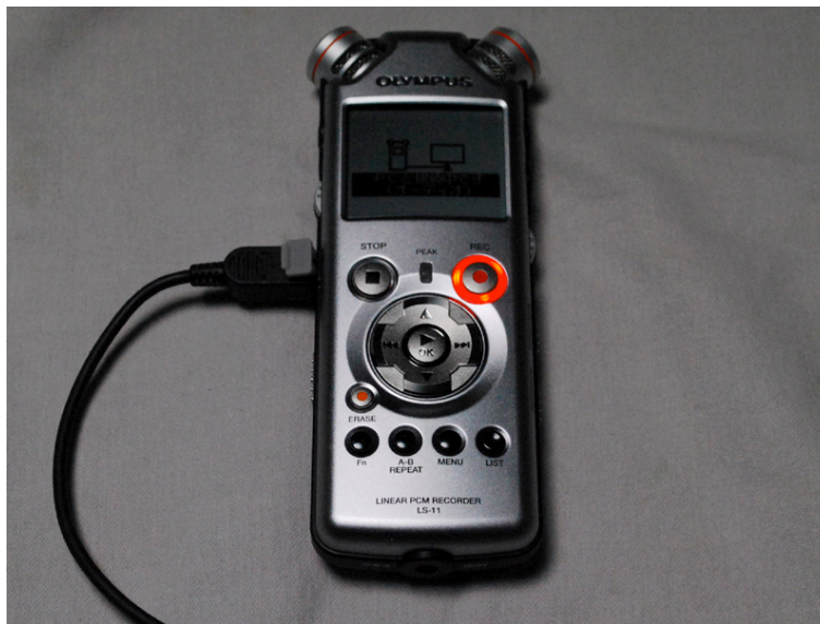
Figure 3.1: A portable linear PCM recorder for recording snoring sounds (Olympus LS-11)
