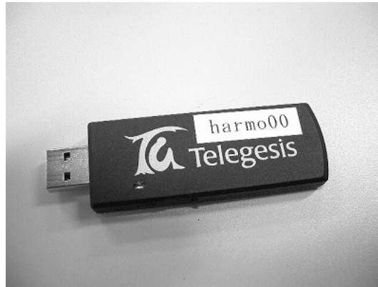
Figure 2.2: ZigBee node, ETRX2USB.
