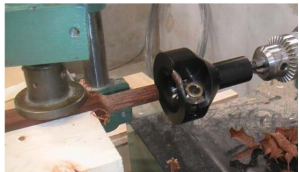
Fig. 4. Cutting a tenon using a tenon cutter mounted on a horizontal drill press.
