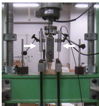
Fig. 6. Withdrawal test for T-type specimens. Note: Arrows indicate locations of the displacement sensors.
