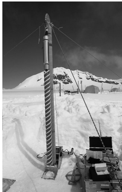
Fig. 3. Drilling system of ILTS used at Mount Wrangell.
