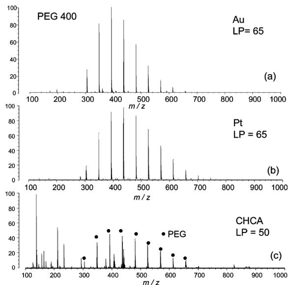
Fig. 5 Mass spectra of polyethyleneglycol, PEG400 (1 mg/mL) obtained using (a) Au nanoparticles, (b) Pt nanoparticles as SALDI matrixes and (c)  $\alpha$ -cyano-4-hydroxycinnamic acid (CHCA) as a MALDI organic matrix (circle indicated peaks: from PEG).
