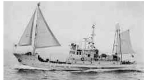
Fig.4 Sail-equipped fishing boat “Enoshima-Maru” (GT: 160, Sail area: 73m<sup>2</sup>)
