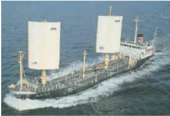
**Fig.6** Sail-assisted tanker “Shin-Aitoku-Maru” (DWT: 1600, Sail area: 200m<sup>2</sup>)
