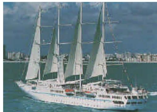
Fig.3 Modern sail-equipped cruising ship “Wind Star” (GT:5703, Sail area:2005m<sup>2</sup>)
