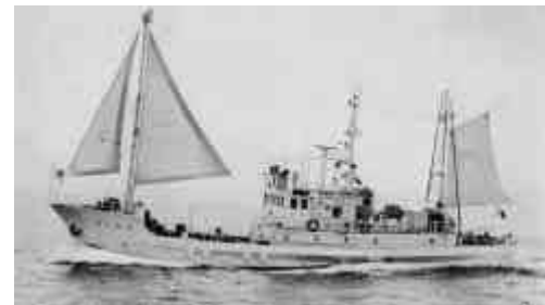
Fig.4 Sail-equipped fishing boat “Enoshima-Maru” (GT: 160, Sail area: 73m 2 )
