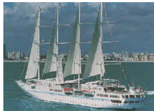
Fig.3 Modern sail-equipped cruising ship “Wind Star” (GT:5703, Sail area:2005m 2 )
