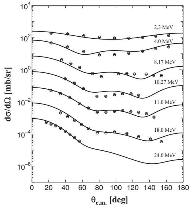
FIG. 10. Elastic angular distribution of the  $n + {}^7\text{Li}$  scattering for incident energies between 2.3 and 24.0 MeV. The solid lines and open circles correspond to the calculated results and experimental data [15,23,27–29], respectively. The data are subsequently shifted downward by a factor of  $10^{-1}$ – $10^{-6}$  from 4.0 to 24.0 MeV.
