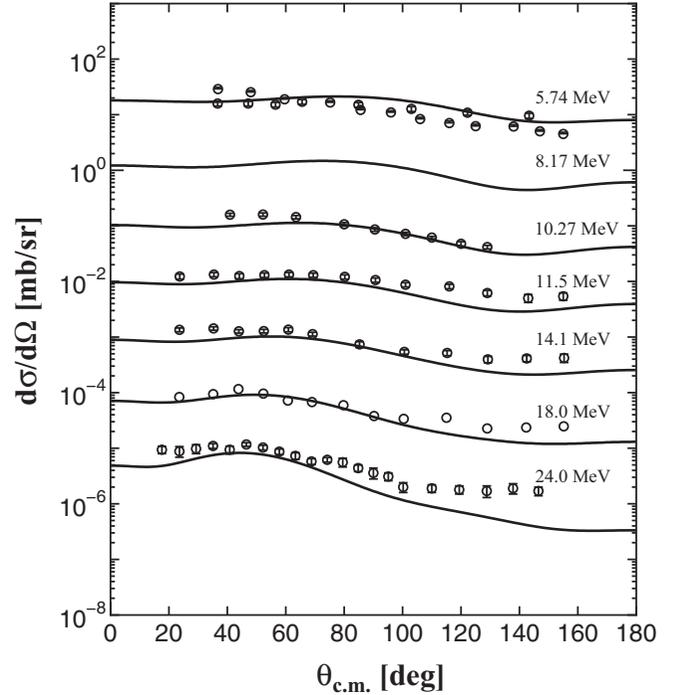
FIG. 6. Angular distributions of the  $n + {}^6\text{Li}$  inelastic scattering for the excited  $3^+$  state at the excitation energy of 2.18 MeV of  ${}^6\text{Li}$ . The solid lines and open circles correspond to the calculated results and experimental data [15,23,25,27–29], respectively. The data are subsequently shifted downward by a factor of  $10^{-1}$ – $10^{-6}$  from 8.17 to 24.0 MeV.
