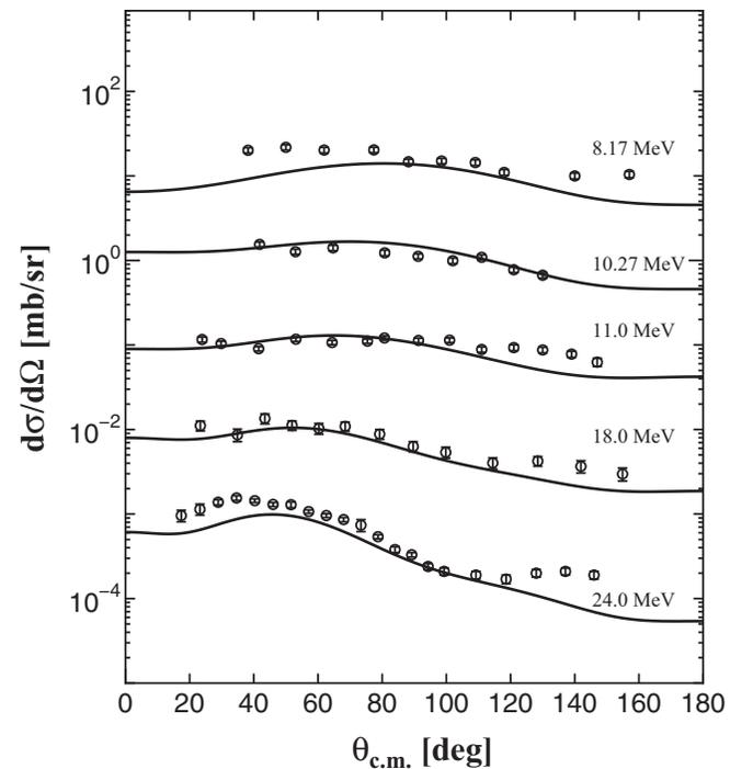
FIG. 11. Angular distributions of the  $n + {}^7\text{Li}$  inelastic scattering for the excited  $7/2^-$  state at the excitation energy of 4.65 MeV of  ${}^7\text{Li}$ . The solid lines and open circles correspond to the calculated results and experimental data [15,23,27,28], respectively. The data are subsequently shifted downward by a factor of  $10^{-1}$ – $10^{-4}$  from 10.27 to 24.0 MeV.
