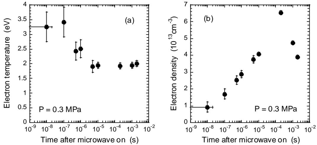
**Fig. 4** Temporal evolutions of (a) the electron temperature and (b) the electron density after the initiation of the microwave power. The helium pressure was 0.3 MPa.
