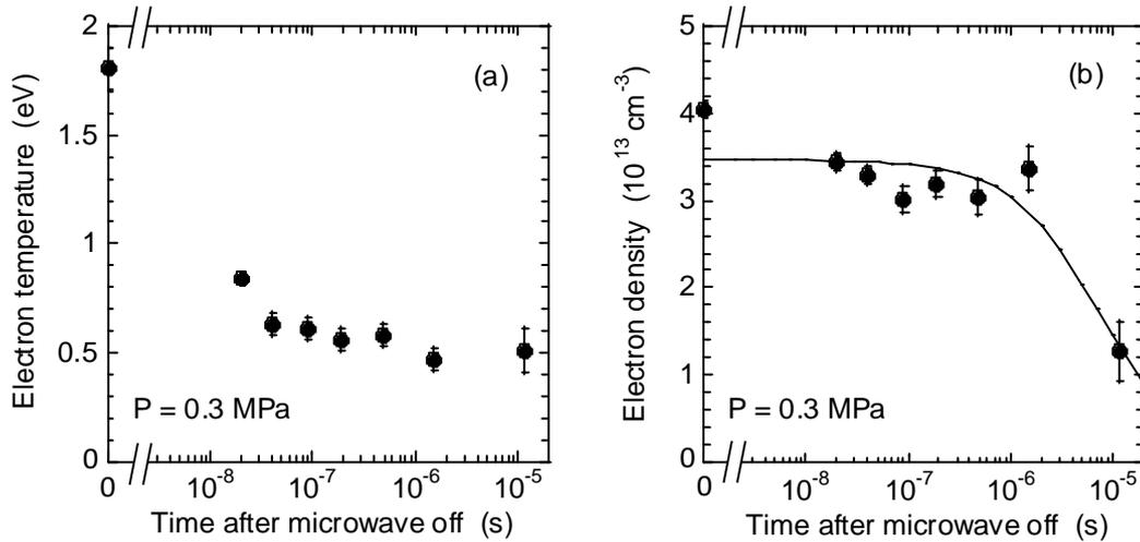
**Fig. 5** Temporal decays of (a) the electron temperature and (b) the electron density after the termination of the microwave power. The helium pressure was 0.3 MPa.
