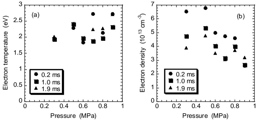
**Fig. 3** Pressure dependences of (a) the electron density and (b) the electron temperature. Values observed at three delay times after the initiation of the microwave power are plotted.
