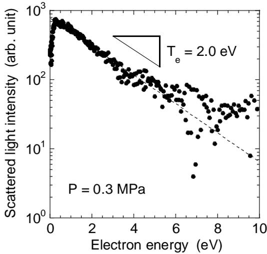
**Fig. 2** Typical electron energy distribution function measured by laser Thomson scattering in a microwave helium plasma at a pressure of 0.3 MPa.
