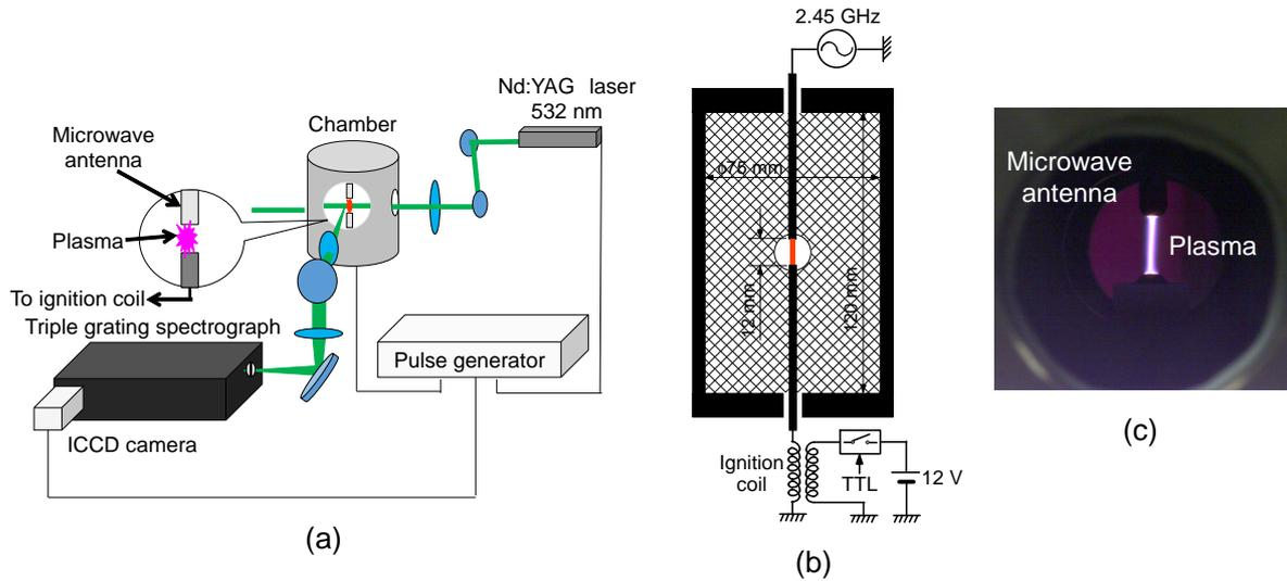
**Fig. 1** Experimental apparatus: (a) schematic of the entire experimental system including the plasma source and the system of laser Thomson scattering, (b) details of the plasma source, and (c) picture of the microwave helium discharge.
