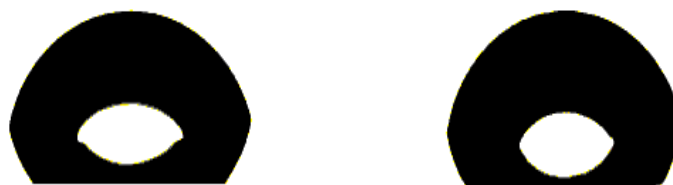
Fig. 2 Reversible switching of contact angle of photoresponsive compound of 1a for water before irradiation (left) and after 366 nm light irradiation (right).
