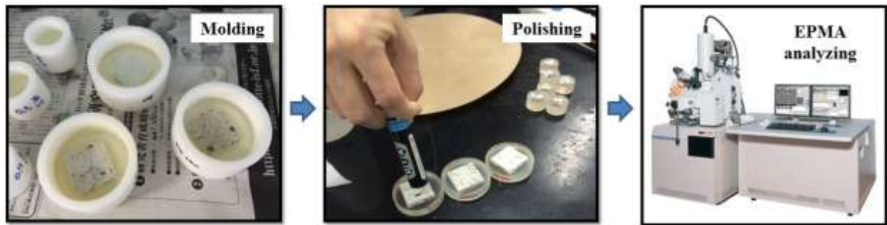
Fig. 3.4 Sample preparation for EPMA
