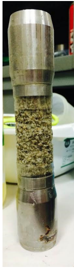
Fig. 5.5: Sample preparation before conducting UCS test.
