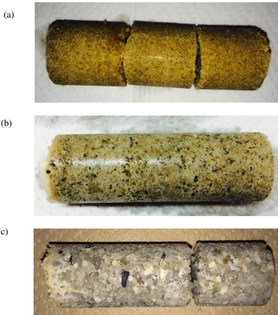
Fig. 4.20: (a) Solidified sample with Mikawa sand, (b) solidified sample with Toyoura sand and (c) solidified sample with Mizunami sand.
