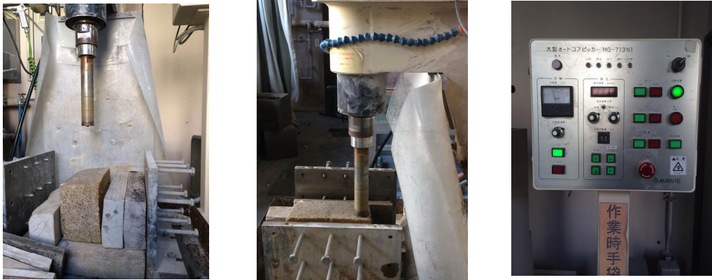
Fig. 5.3: Procedure for sample coring using rock coring machine.
