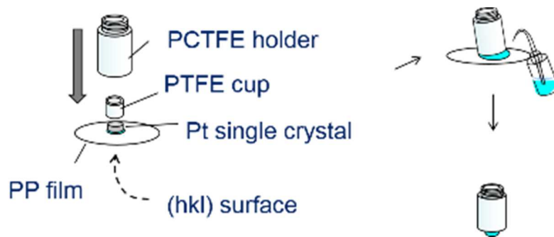
Fig.2.2.4 Schematics of the embedding of an electrode into an RDE assembly.
